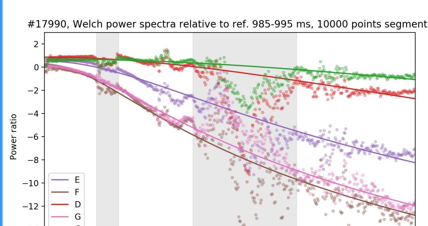
Frequency response comparable to first order filter: only shielding effect
