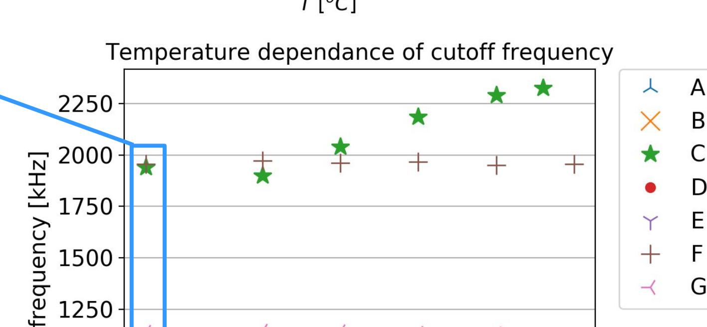
Capacitance and frequency response approximately constant for temperatures relevant for the first phase of COMPASS-U operation. Resistance scales linearly and can double at 300 °C
